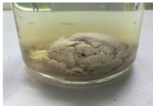
Glue to which no glutaric aldehyde was added after 24 h of soaking in water
