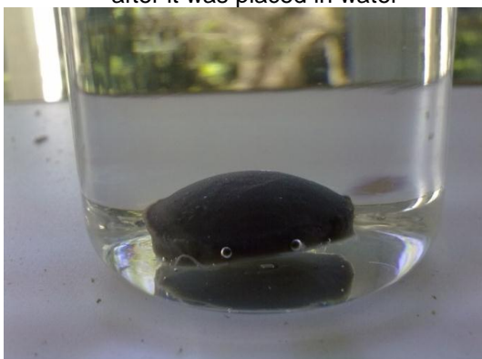
Control sample without transglutaminase treatment just after it was placed in water
