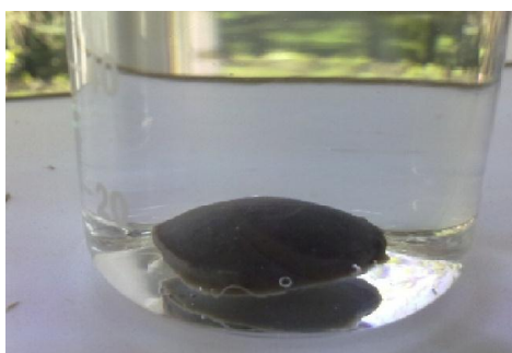
Glue to which 1.2 mL of 5% glutaric aldehyde were added just after it was placed in water
