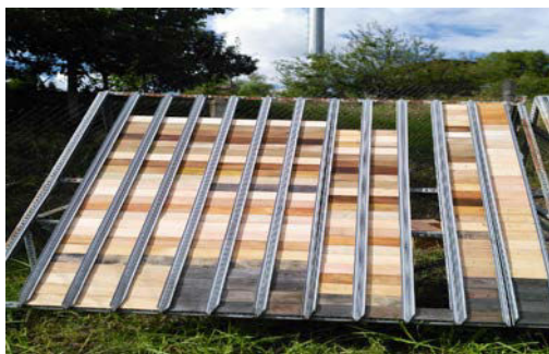
Figure 1. Weathering rack in Bartın province
