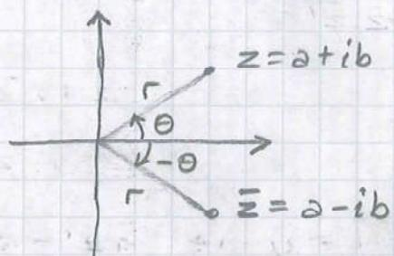
$$\begin{aligned} \bar{z} &= a-ib = r \cos \theta - r \sin \theta = r(\cos \theta - i \sin \theta) \\ &= r(\cos(-\theta) + i \sin(-\theta)) \end{aligned}$$
