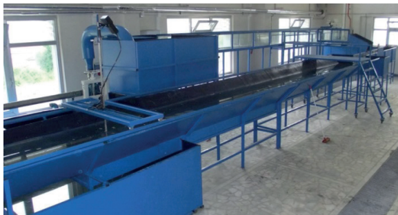
Figure 3. Open channel structure
