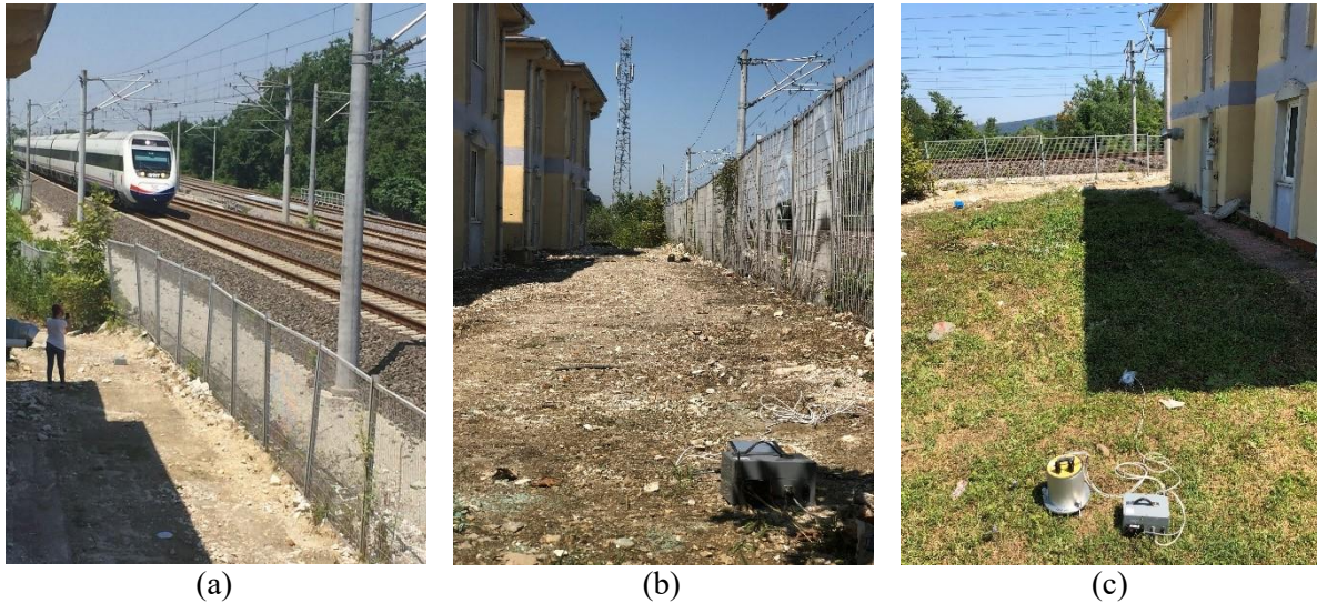
Figure 2. Field view and installation of accelerometers.
