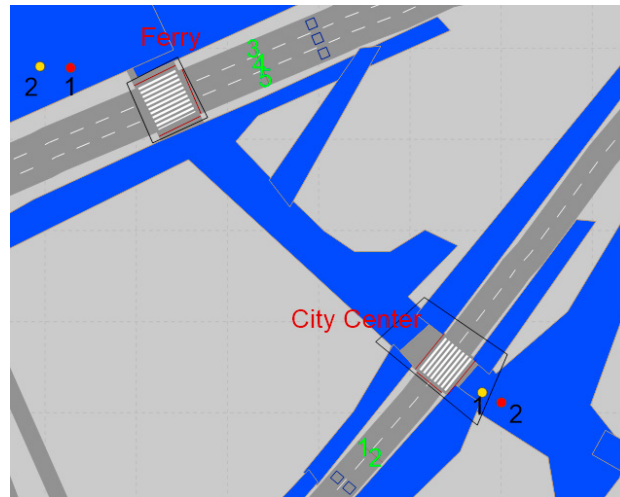
Fig. 3. Intersections considered in case area at VISSIM environment.
