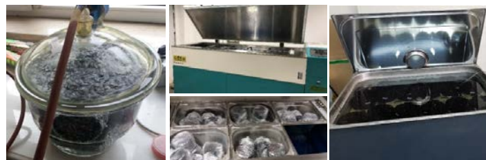
Fig. 3. Conditioning stages (vacuuming, freeze-thawing and heating in a water bath) of moisture susceptibility test sample
