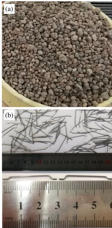
FIGURE 1 Expanded clay as coarse aggregate (a) and hooked steel fiber (b)
