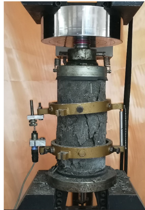
FIGURE 9 Modulus of elasticity setup
