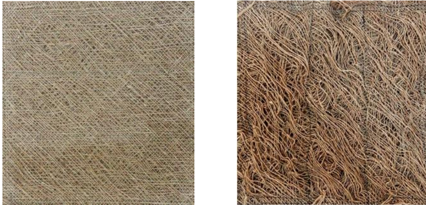
Figure 2. Untreated and treated nettle fibre yarns
