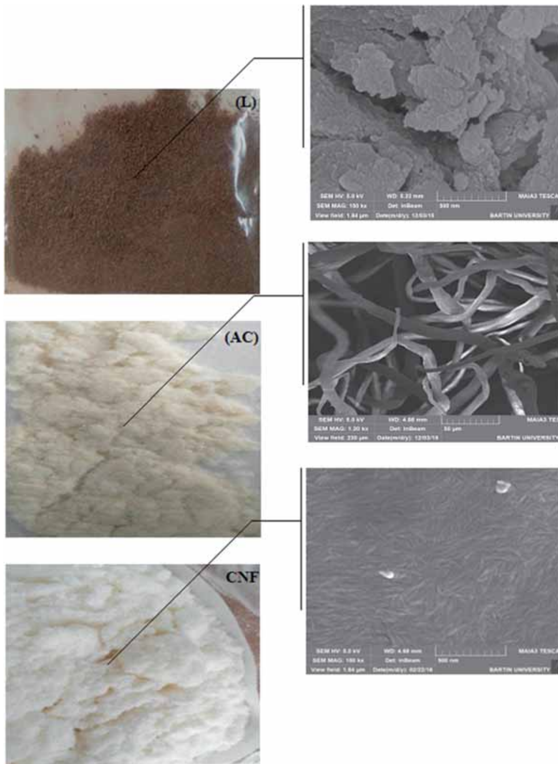
Figure 1. Scanning electron microscopy images of the reinforcing fillers.
