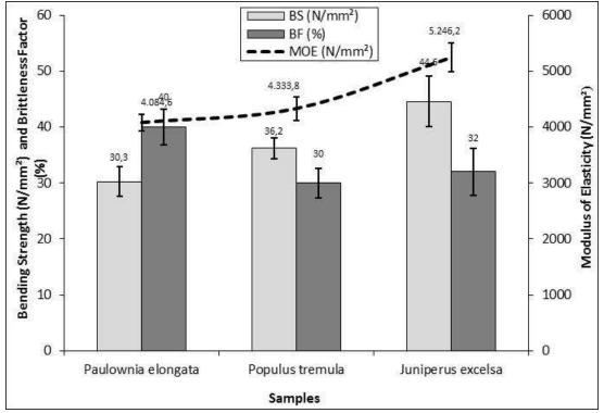
**Fig. 2.** Mean estimates for bending strength (BS), modulus of elasticity (MOE), and brittleness factor (BF)
