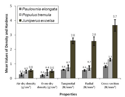
Fig. 1. Mean values of density (air-dry and oven-dry) and Brinell hardness (tangential, radial, and cross-sectional)
