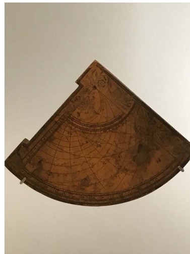
Figure 4. Ottoman, 17th c. Astrolabe Quadrant (Musee IMA inv. Al 84-08). Assume that an observer stands on the south pole and there exists a tangent plane in the north pole, the 1/4th of the conical projection of the sky to that mentioned plane called Astrolabe Quadrant. That device is widely used for astronomical calculations and time keeping until the beginning of 20th century. It also calculates longitude of Sun.
