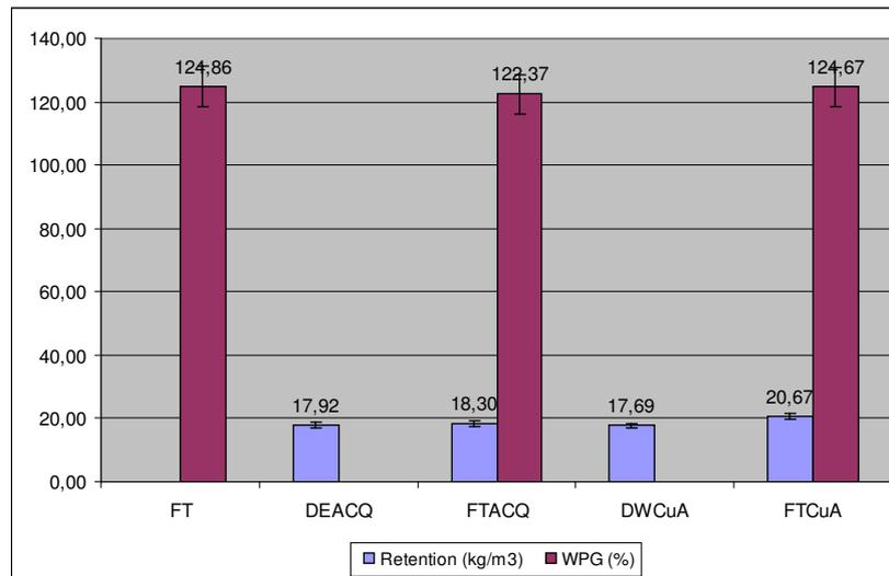
Figure 2. Retentions (kg/m<sup>3</sup>) and weight per cent gain (%) of samples
