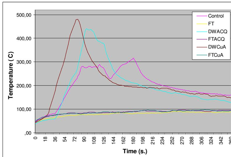
Figure 4. Maximum temperature of wood during the test
