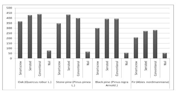
Figure 1. The histogram of nail-screw withdrawal resistances for radial direction.
