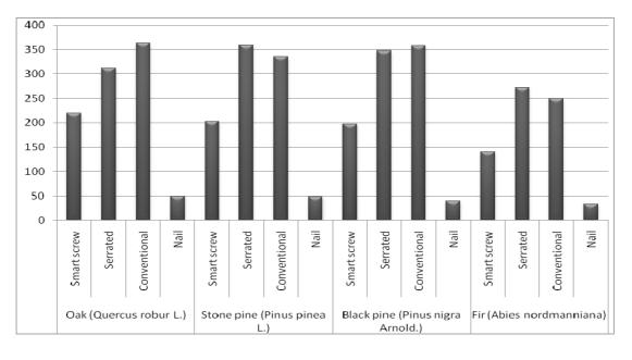
Figure 3. The histogram of nail-screw withdrawal resistances for longitudinal direction.
