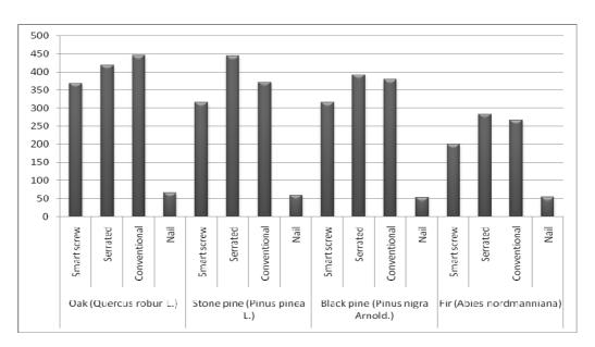
Figure 2. The histogram of nail-screw withdrawal resistances for tangential direction.
