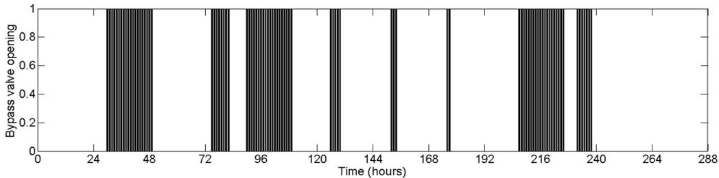
**Figure 9.** Operational scheduling for the bypass valve of the single NC 100–200 turbine installed at location 4.
