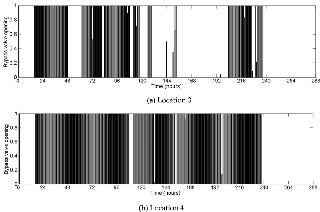
**Figure 12.** Operational scheduling for the bypass valves of the two NC 150–200 turbines installed at locations 3 and 4.
