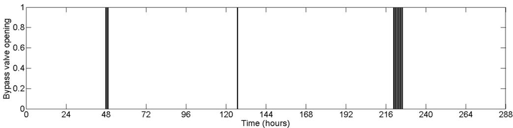
**Figure 10.** Operational scheduling for the bypass valve of the single NC 150–200 turbine installed at location 4.
