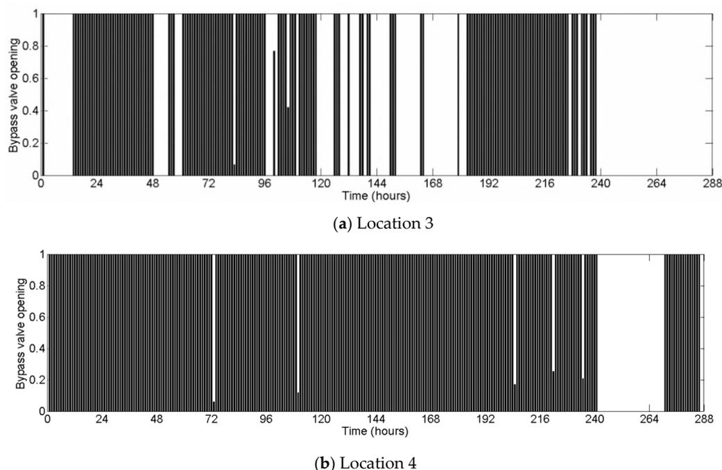
**Figure 11.** Operational scheduling for the bypass valves of the two NC 100–200 turbines installed at locations 3 and 4.
