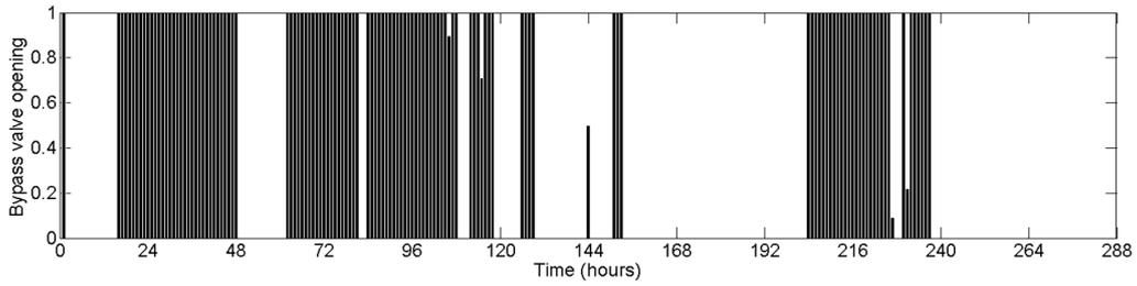
**Figure 8.** Operational scheduling for the bypass valve of the single NC 150–200 turbine installed at location 3.
