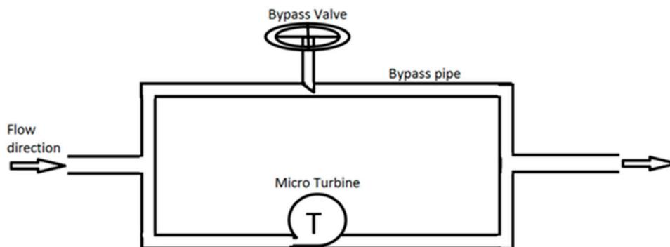
**Figure 1.** Micro turbine/bypass valve combination.
