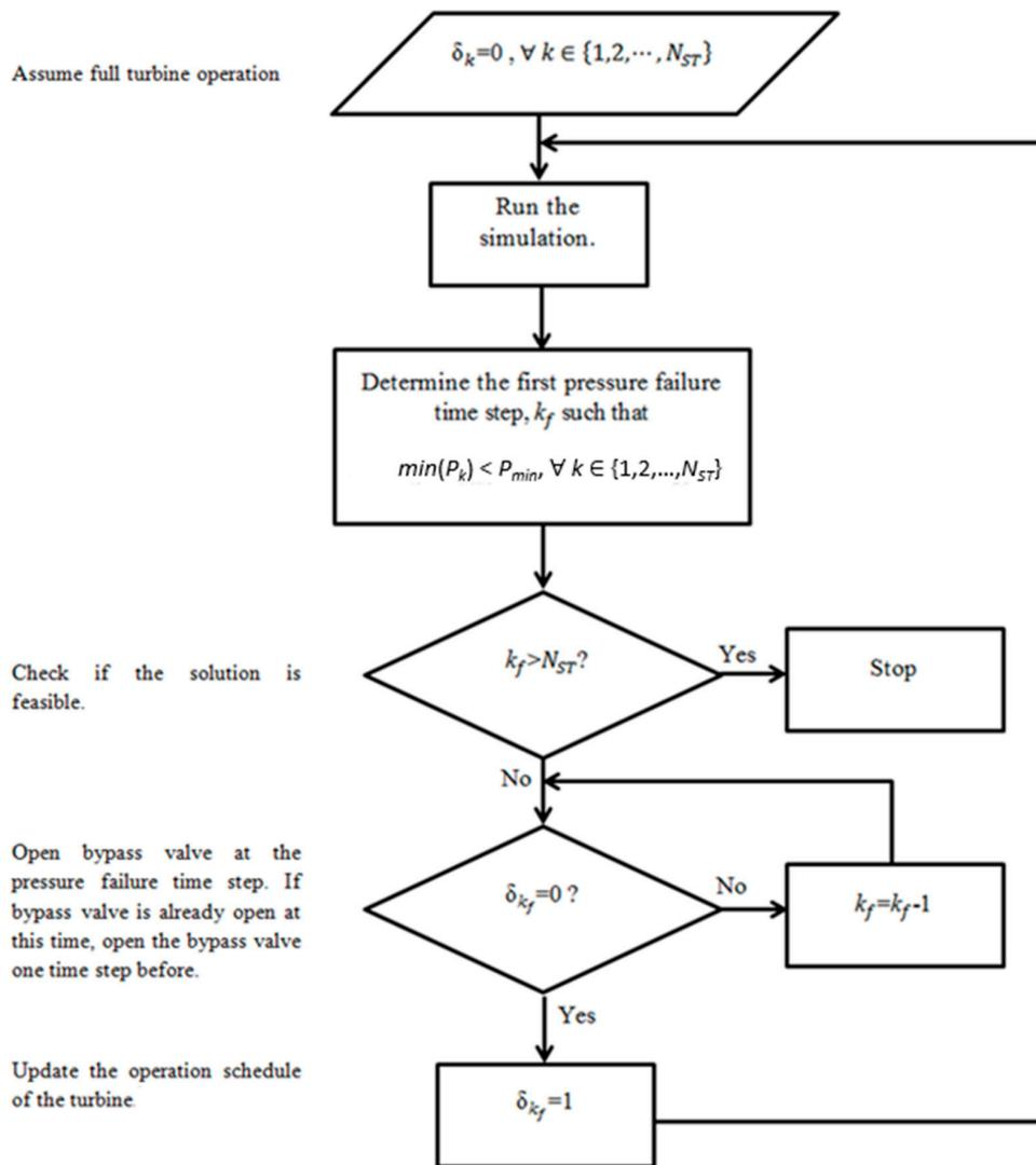
Figure 2. Process of obtaining a smart seed.
