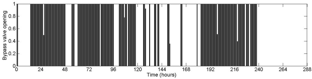
**Figure 7.** Operational scheduling for the bypass valve of the single NC 100–200 turbine installed at location 3.
