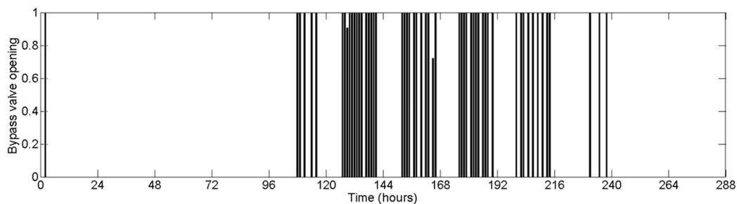
Figure 14. Operational scheduling for the bypass valve of the NC 100–200 turbine installed at location 4.
