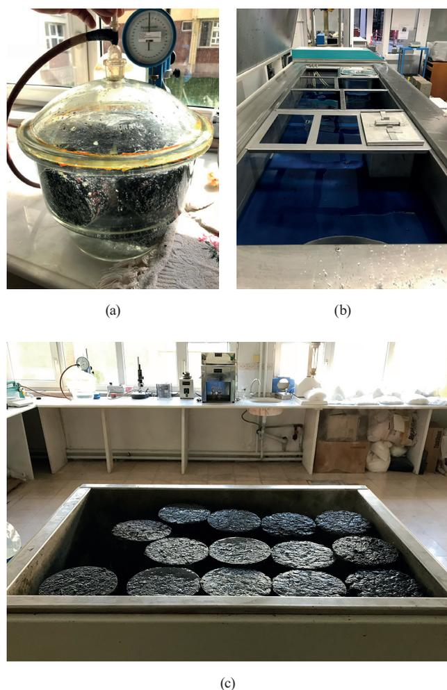
Fig. 4 The conditioning procedure of the specimens, (a) Vacuum application, (b) Freezing step and (c) Heating in a water bath
