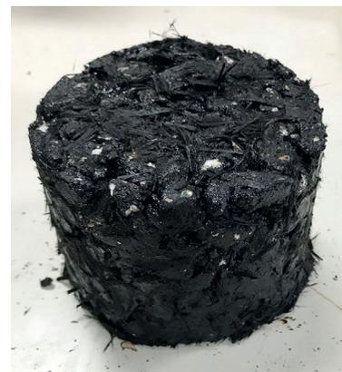
Fig. 9 An excessive heterogeneous matrix due to surplus fiber content
