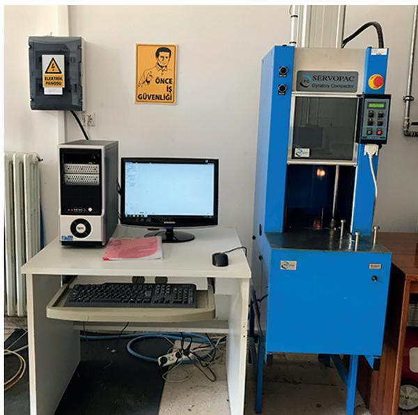
**Fig. 3** Gyrotory compactor
