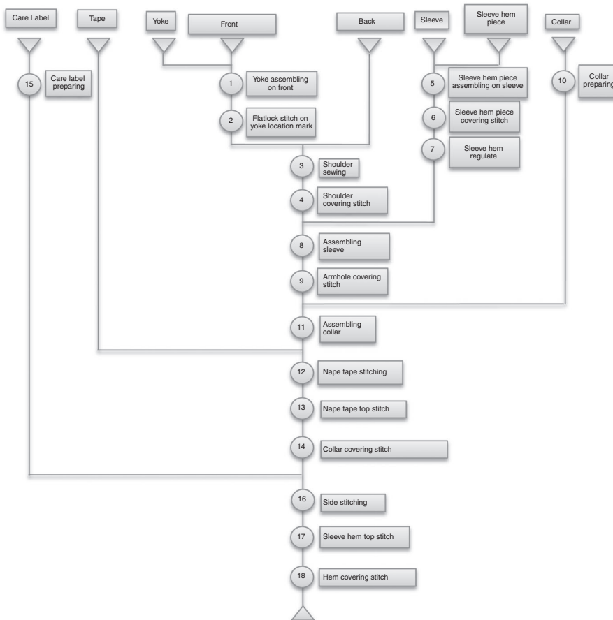
Figure 2. Operations and flow chart of the operations in t-shirt production
