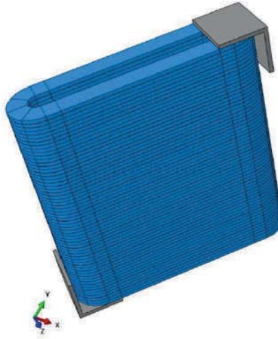
Figure 1. Finite element model of the wall panel and rigid loading plates.
