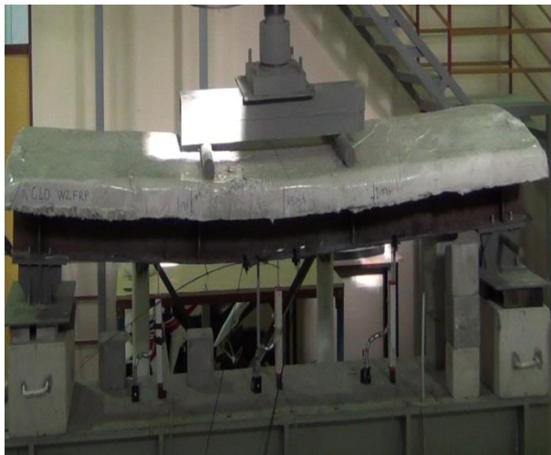
Figure 17. Deformed shape of the strengthened sample
