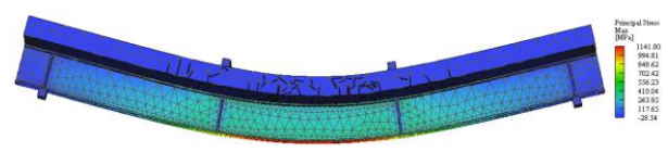
Figure 23. Principle stress contour and cracks in strengthened with two layers of CFRP steel-concrete composite beam (CBW2 CFRP)
