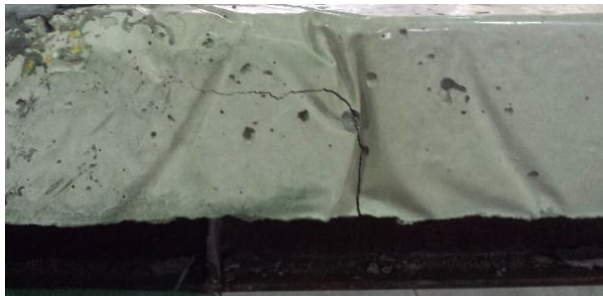
Figure 12. Shear cracks of the CW0CFRP sample
