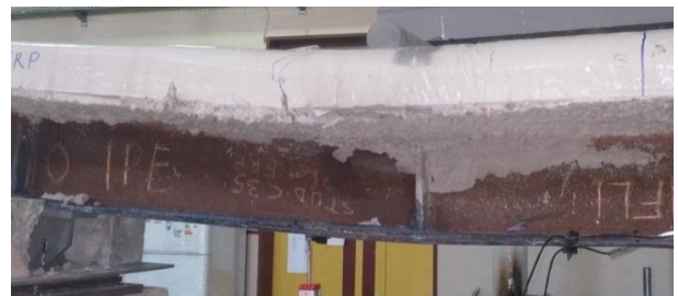
Figure 20. Concrete crushing and deflection of CBW3CFRP sample
