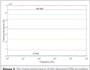
**Figure 5.** The transconductance of the designed OTA according to the biasing currents
