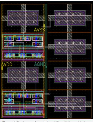
Figure 6. The layout of the designed filter (30.2  $\mu m \times 35.45 \ \mu m;$  0.00107  $mm^2)$
