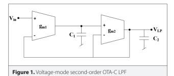
Equations (2) and (3) give the resonance frequency ( $\omega_o$ ) and quality factor (Q), respectively.
