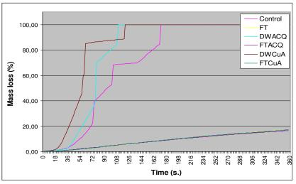
Figure 3. Mass loss course during the test
