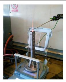
Figure 1. The appearance of test machine and the sample burning
