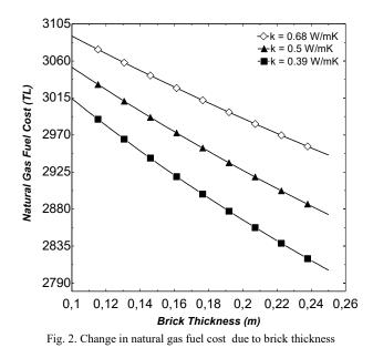
Here, the annual natural gas fuel cost is expressed in TL. As can be seen, when comparing according to the change of the brick thickness, the natural gas fuel cost corresponding to each thickness is less in clay bricks made of wastes.
