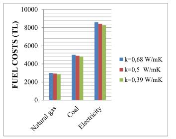
Fig. 5. Change in natural gas, coal and electricity fuel cost due to brick thickness
