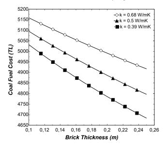
Fig. 3. Change in coal fuel cost due to brick thickness
