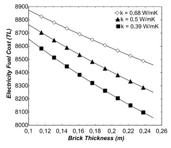
Fig. 4. Change in electricity fuel cost due to brick thickness
