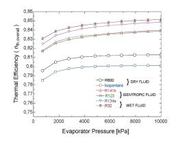
Figure 2. Exchange of overall thermal efficiency with Evaporator Pressure
