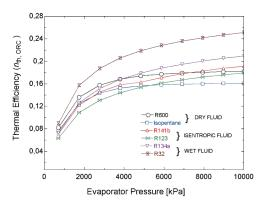
Figure 3.Exchange of ORC thermal efficiency with Evaporator Pressure
